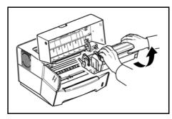
3 Using the green handles lift the *Drum Unit* out of the machine.
